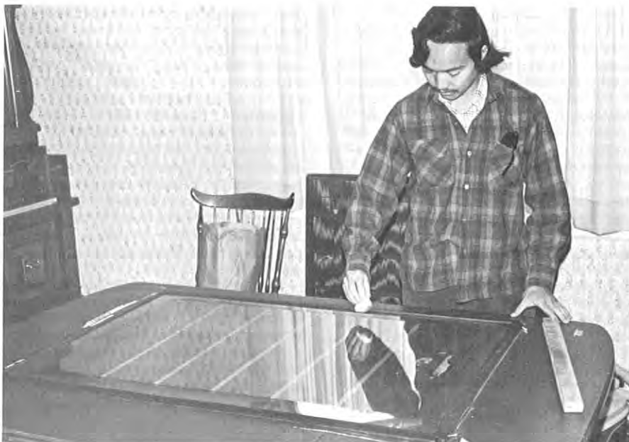
Photo two, at left, is a closeup of two panels of the piano wire type installed in oak frames and wires attached. A friend of the author's, below, rubs in some graphite on a stretched mylar diaphragm.
